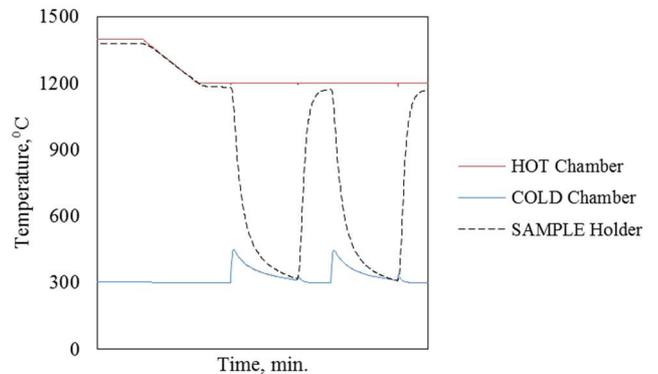
Figure 2 - Example of temperature profiles recorded during a cyclic thermal shock test with initial pre-treatment.
