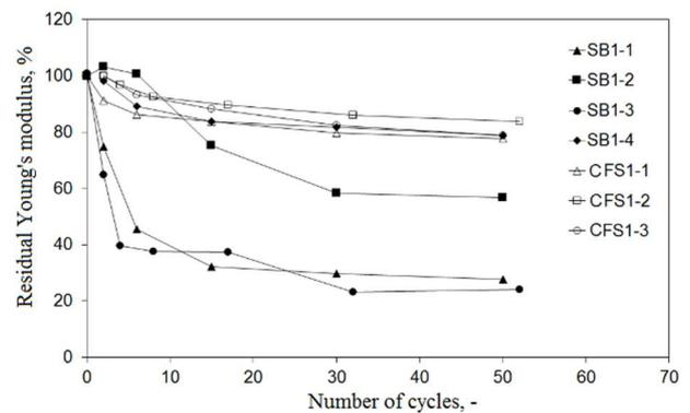
Figure 3 - Change of Young's modulus with thermal cycles in the samples of two materials.
