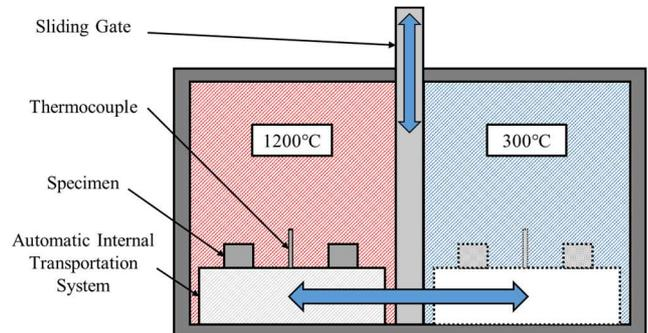
Figure 1- Schematic of the testing equipment [2].
