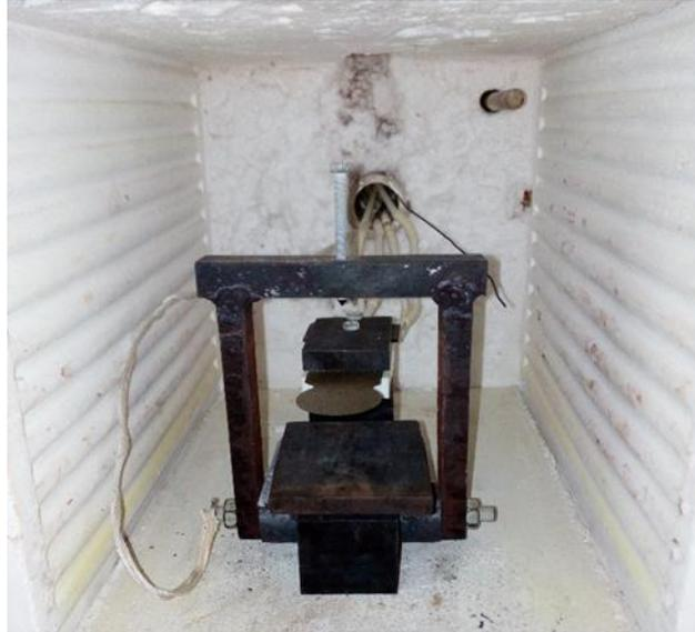
Figure 3: Hot disk device for medium temperature measurements.
