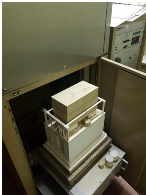
Figure 4: Hot wire device for high temperature measurements.
