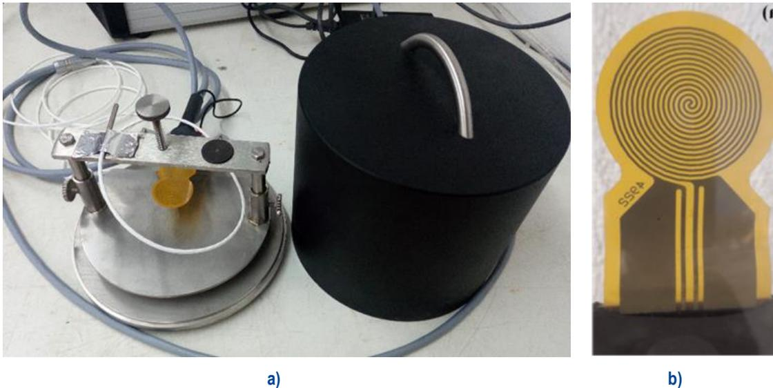
Figure 2: a) hot disk device for room temperature measurements; b) TPS sensor.
