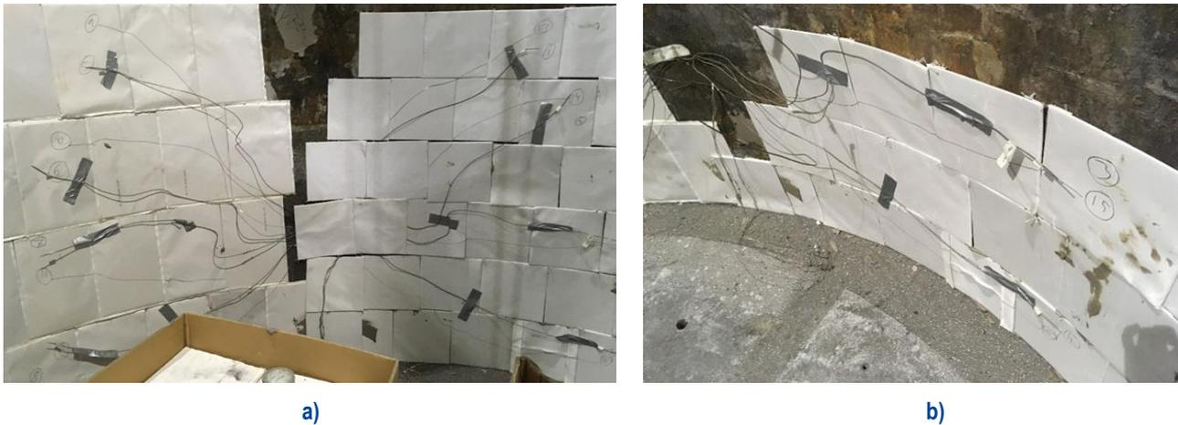
**Figure 7: Installation of thermocouples on steel ladle lining: a) front view; b) top view.**
