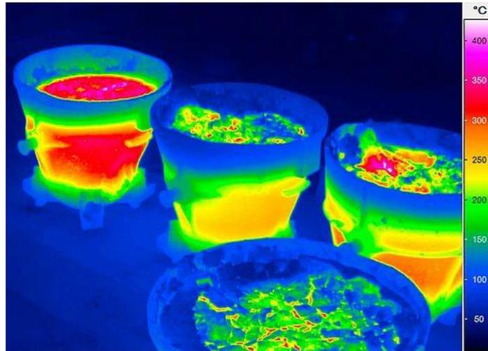
Figure 8: Example of an infrared image of four full steel ladles.
