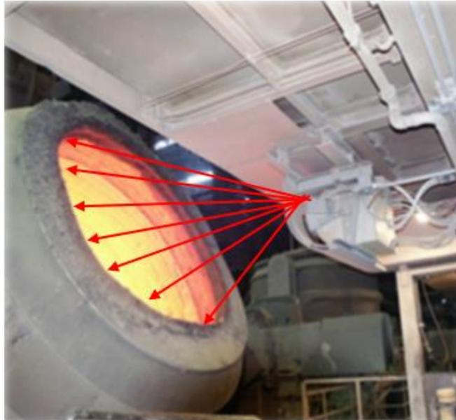
**Figure 9: Laser scanner measures on the internal surface of the ladle from the outside the steel ladle**
