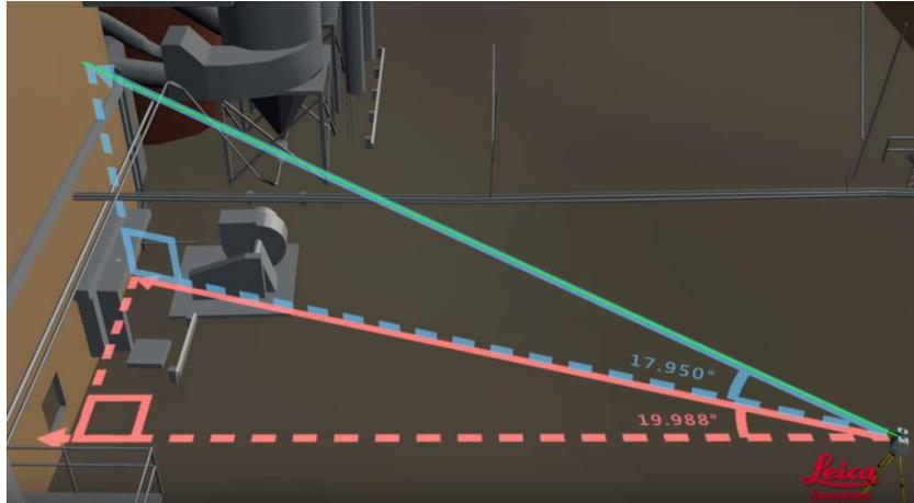
**Figure 4: Vertical and horizontal angles (Source: Leica Geosystems).**
