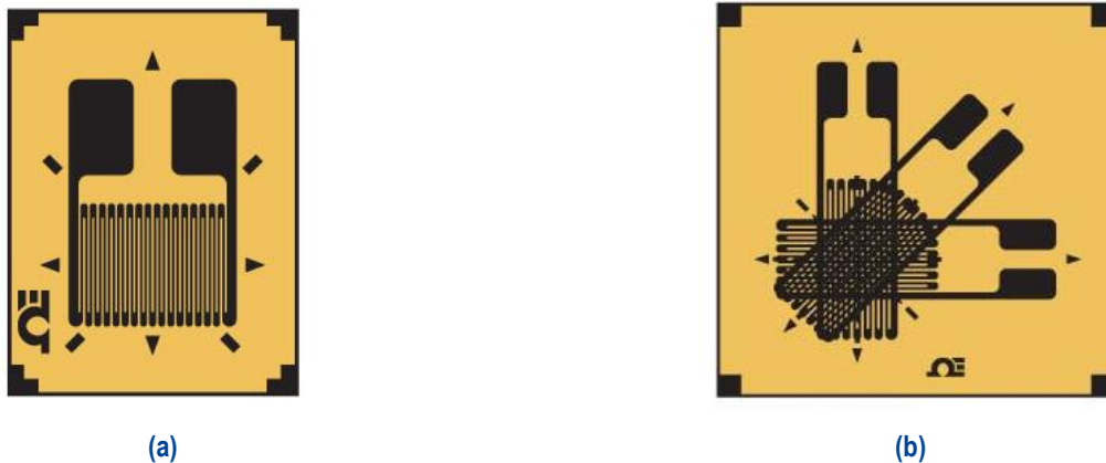
Figure 6: Resistive strain gauges: (a) Uniaxial strain gauge; (b) Triaxial strain gauge
