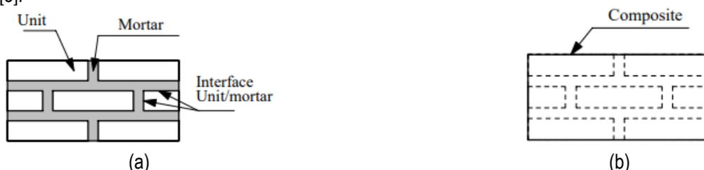
**Figure 1 - Modelling strategies for masonry structures [3]: (a) micro-modelling; (b) macro-modelling**
