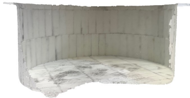
Figure 45 - Example of photogrammetry on the inner surface of the pilot ladle in its current state.
