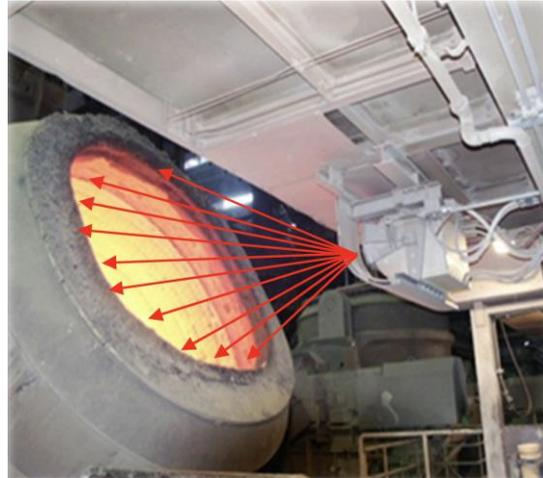
**Figure 7 - Example of laser scanner measures from outside position [5].**
