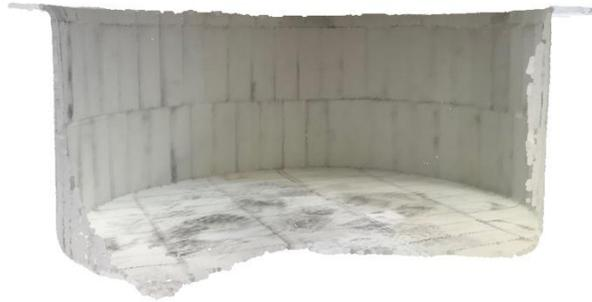
**Figure 10 - Example of photogrammetry (lining of Pilot steel ladle).**
