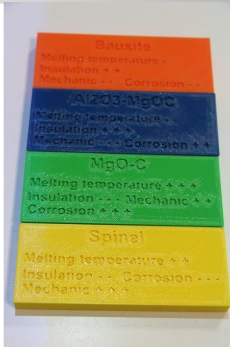
Figure 4: 3D-printed refractory bricks, with simplified technical information.
